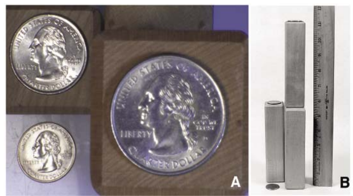
Figure 5. A: Image taken with a 600CL of US quarters on blocks of wood. The image was levels adjusted and sharpened in Adobe Photoshop. The camera was focused on the middle quarter with the Computar iris at f 5.6 and the image taken at an f-stop slightly above "+" (i.e., more than one f-stop above 32, see Fig. 4). Image depth of field/field width is approximately 3.5. B: Side view of the same objects shown in A. Approximately 140 mm (5 1/2 inches) separate each quarter for a total depth of field of more than 280 mm (11 inches).
