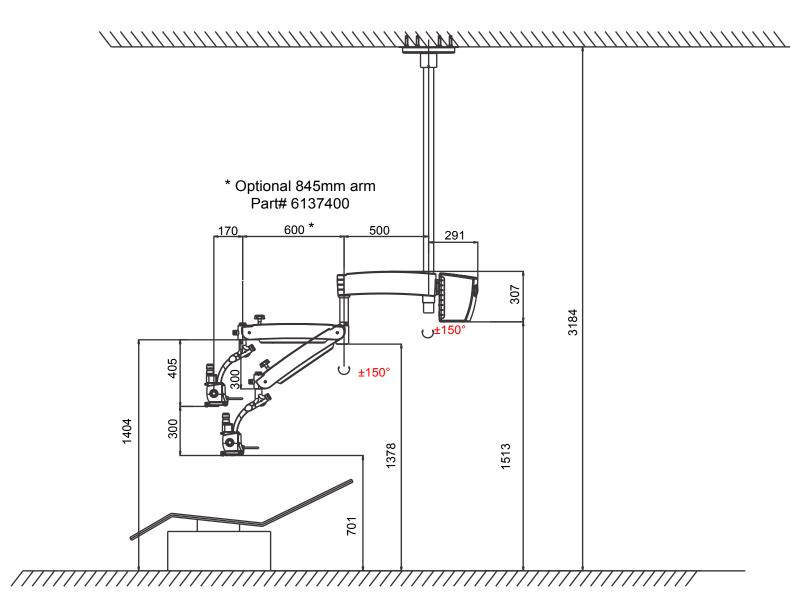
Note: Use of optional 845mm suspension arm requires longer fiber optic cable (part# 6165000-380)
